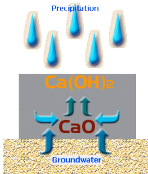
This soluble Calcium Hydroxide can migrate to the surface of the paving, whereupon it has the opportunity to react with Carbon Dioxide (CO<sub>2</sub>) in the
